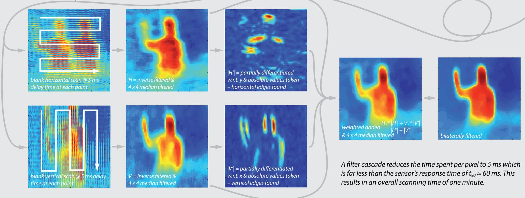
A filter cascade reduces the time spent per pixel to 5 ms which is far less than the sensor's response time of  $t_{90} \approx 60$  ms. This results in an overall scanning time of one minute.
