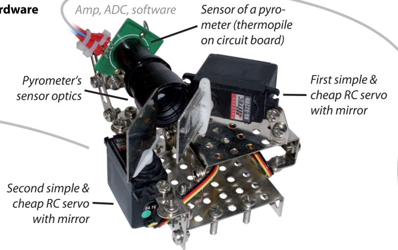
Metallic objects reflect infrared light, but do not themselves emit infrared light according to their temperature (Kirchhoff's law). That enables this simple prototype.
